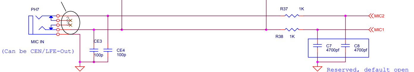
Analogue I/O connection of the ALC650
